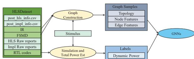
Fig. 4: Usage of HLSDataset to construct machine learning based power model
