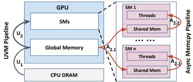
Figure 1: CPU-GPU system data transfer pipeline. With *UVM*, the pipeline contains  $U_1$  and  $U_2$  stages. Adding *Async Memcpy* atop of *UVM*, stage  $U_2$  can be pipelined into  $A_{2.1}$  and  $A_{2.2}$ .
